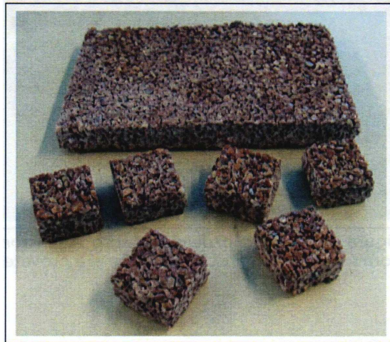
Image 1.1 - Floor section Aquastone Marmorite with crushed grain size 2-6 mm and specimens.
