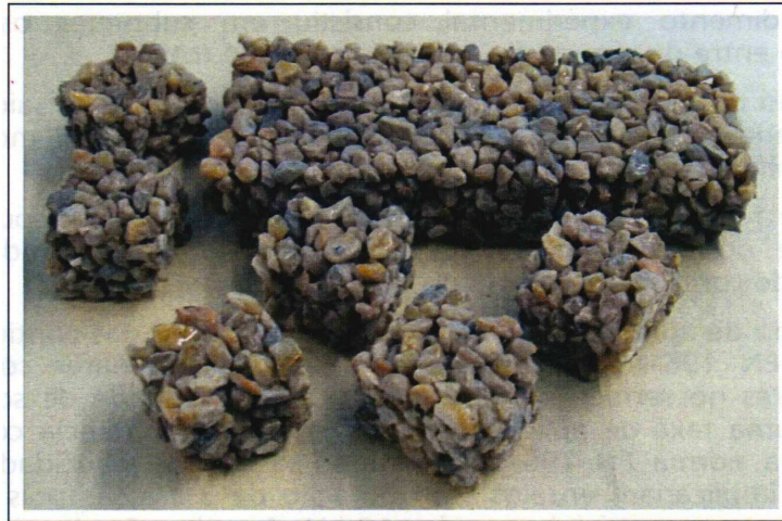
Image 1.3 – Section Aquastone boulder pavement with grain size 4-8 mm and specimens..
